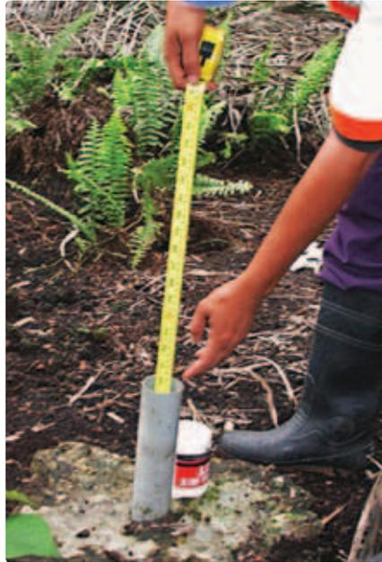
Figure 7-6: Example of piezometer for measuring groundwater levels.
