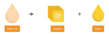
**Fractionation** - involves the splitting of oil into parts or fractions. This can be repeated to obtain several fractions from one raw material. In palm oil and palm kernel oil the fractionation process normally fractionates to six different levels. It is possible to fractionate to further levels for functionality. This is achieved by cooling the oil under controlled conditions (crystallisation) and filtering. In short, the liquid palm olein is separated from the solid stearin.
