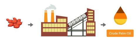
Fresh fruit bunches (FFB) are delivered to a mill from large plantations, traders and smallholders. FFBs are sterilised and stripped. The fruit is pressed to separate the oil from the kernel. The oil is purified and clarified.
