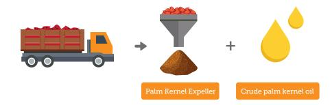
Palm Kernels are transported to separate crushing facilities. The kernel is cracked and removed from the palm kernel shell, which is used as biomass fuel. The kernel is crushed to produce palm kernel oil(PKO) and palm kernel expeller (PKE).
