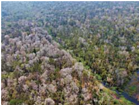
Figure 3-34a (above) and 3-34b (right): Peat swamp forest trees killed by elevated water levels caused by back-flooding of the forest as a result of the construction of adjacent bund with no culverts between the forest and agricultural land.
