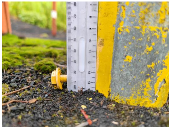
Figure A3.3: Photo showing measurement rule to read subsidence level.
