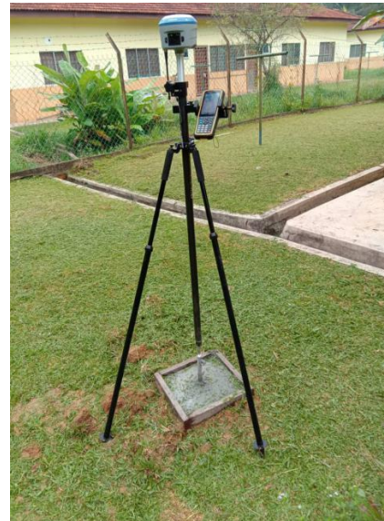
Figure A5.4: Observation of Temporary Benchmark
