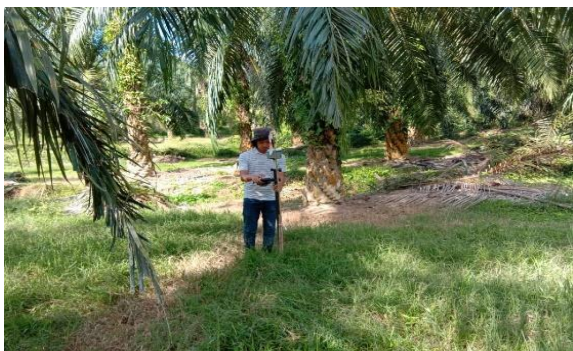
Figure A5.5: Spot height measurement using GPS Rover
