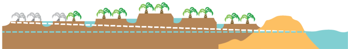
Figure 5: As the soil subsides, occurrence of flooding is witnessed in area closer to NDL
