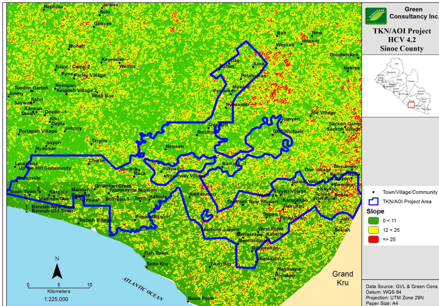
Figure 7: HCV 4.2 Map depicting slope across the AOI. Areas that are 12-25 degrees in slope (yellow) should be terraced, while areas >25 degrees in slope (red) should not be planted. Areas in green are relatively low risk for erosion.
