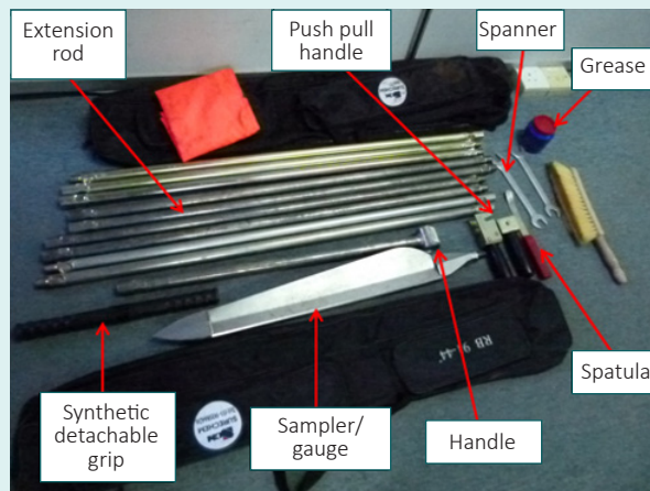
Figure 2: Peat auger tools and method to use this auger (Credit: Global Environment Centre, GEC)
