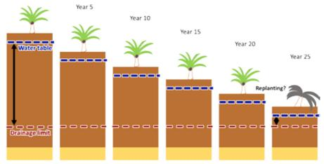
Figure 3-22: How peat soil subsidence impacts the depth to the drainage base (natural drainage limit). Over time, the peat layer above the drainage base may become too shallow to permit replanting.
