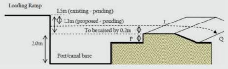
Figure 3-18: Alteration made to existing spillway crest (increasing the height to reduce over drainage).
