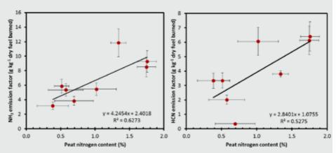
Figure 2-9: Scatter plots showing the relationship between peat substrate peat nitrogen content and ammonia (left) and hydrogen cyanide (right) emission factors. A linear regression line of best-fit is presented (solid black line). Both lines of best-fit have a statistically significant non-zero slope (p<0.05).
