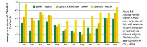
In droughts, the water level can drop 0.5- 1cm per day. During a one month drought the water level may fall 15-30cm if there is no input from surface or sub-surface flow. Therefore in areas with extended dry seasons it is recommended to raise the water levels in the plantation as high as possible at the end of the wet season – so that in subsequent dry periods the level can be maintained at 40-50cm in the field.
