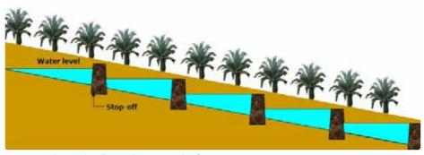
Figure 3-6: Along each collection drain a cascade of weirs is required with one stop-off or weir recommended for every 20cm drop in level.
