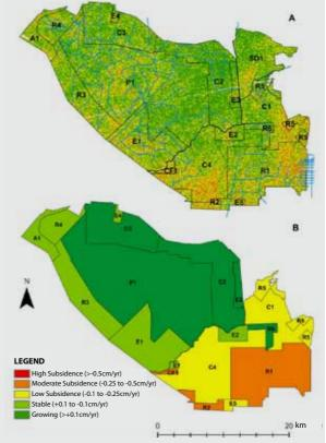
Figure 2-10: A) Average subsidence over each management zone as measured by ISBAS InSAR and associated indicative subsidence risk B) Management designation in the NSPSF Integrated Management Plan and indicative subsidence risk.
