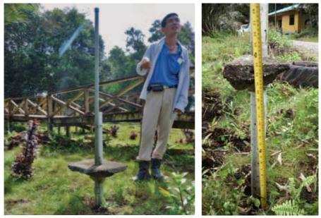
Figure 7-1: Example of subsidence pole installed together with a piezometer [Photograph on the left taken in 2011 and that on the right taken in 2018 for the same pole. Peat subsidence over time in this site is clearly visible.
