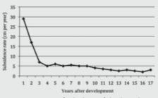
Figure 2-5:Progress of subsidence of the drained peat under oil palm cultivation at the MPOB Research Station, Sessang, Sarawak.
