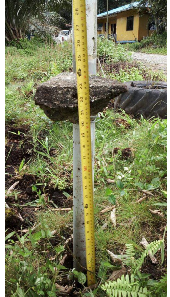
Figure 7-1: Example of subsidence pole installed together with a piezometer [Photograph on the left taken in 2011 and that on the right taken in 2018 for the same pole. Peat subsidence over time in this site is clearly visible.
