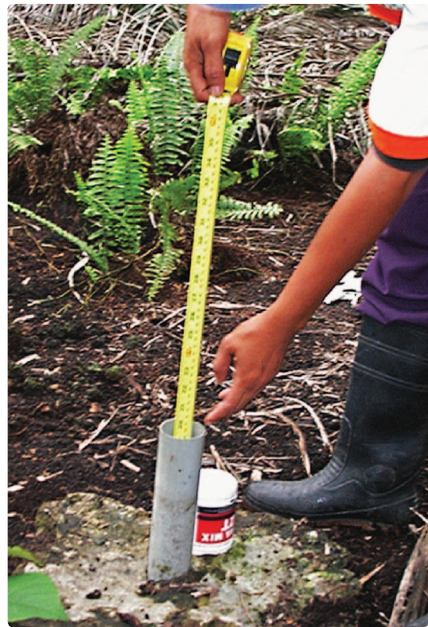
Figure 7-6: Example of piezometer for measuring groundwater levels.
