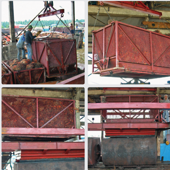
Figure 5-4: Series of photos showing the new system of FFB transportation. From top left: FFB in cages being lifted out of a pontoon, cage being moved and positioned over a boiler cage and FFB emptied into the boiler cage.
