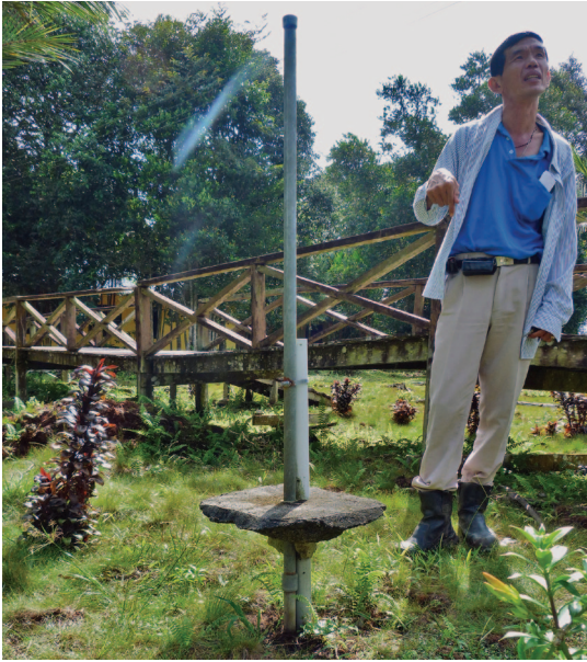
Figure 7-1: Example of subsidence pole installed together with a piezometer [Photograph on the left taken in 2011 and that on the right taken in 2018 for the same pole. Peat subsidence over time in this site is clearly visible.
