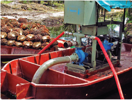
Figure A5-1: Close up example of fire boat used for fire suppression activities in oil palm plantations on peatland.
