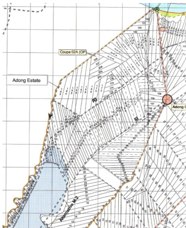
Figure 3-12: The drainage layout for Adong estate in Woodman Plantation, Miri, Sarawak (map on left and satellite image on right). The design of the drainage system is based on the contours with collection drains running along the contour lines at an acute angle to the main or outlet drains.
