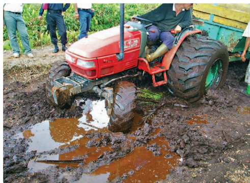
Figure 5-5: Operational problems encountered when ground bearing capacities of deep peat are exceeded.
