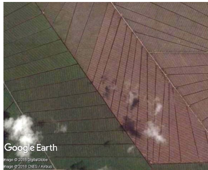
Figure 3-13: Following the contours and setting high water levels along collection drain in Woodman estate in Bintulu, Sarawak enables FFB to be transported by barge pulled by a small boat with a 15hp engine.
