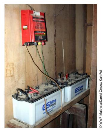
Figure 7. An energizer powered by wet-cell batteries.
