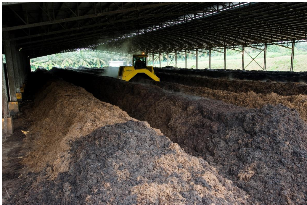
Figure 53. Heavy Equipment is employed to turn Windrows
