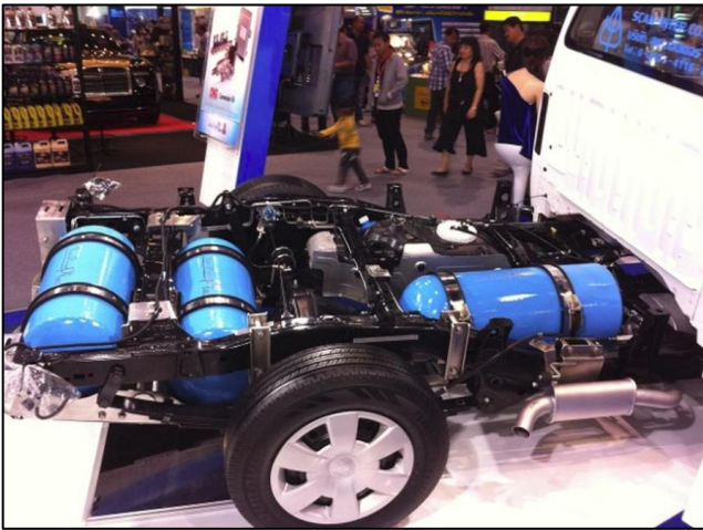
Figure 15. View of fuel storage for truck after conversion from diesel to CNG or liquefied biogas operation.
