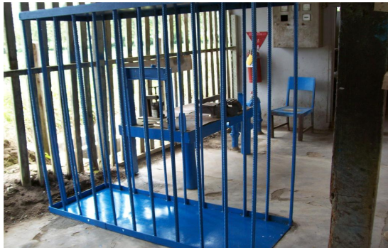
Figure 4 Tyre Cage at all Workshops
