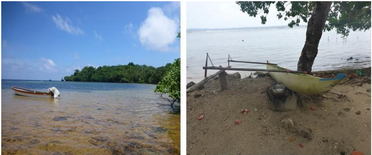
Figure 8: Common vessels used for fishing. Left image and powered, fiberglass 'banana boat', and right image a traditional, outrigger canoe made from Erima ( Octomeles sumatrana ).
