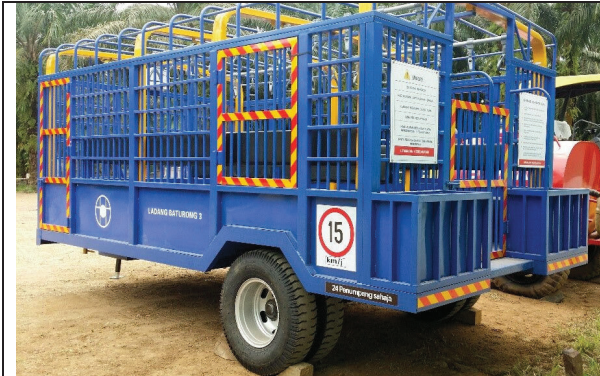
Passenger trailer for transportation of workers at IOI Baturong PMU.
