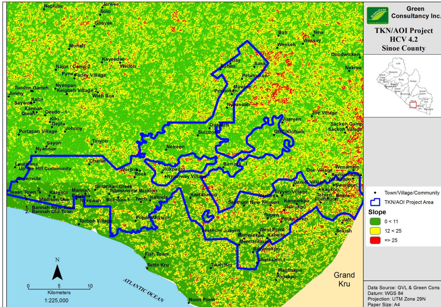
Figure 8: HCV 4.2 Map depicting slope across the AOI. Areas that are 12-25 degrees in slope (yellow) should be terraced, while areas >25 degrees in slope (red) should not be planted. Areas in green are relatively low risk for erosion.
